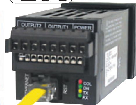
1/16 DIN Controller With Embedded Web Server, Dual Control Outputs, Dual Display
