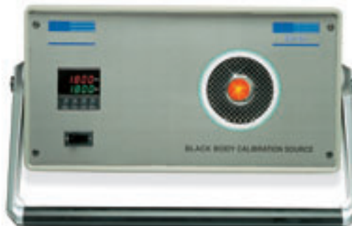
Model BB-4A, $3595 100 to 982°C (212 to 1800°F), .8" (22 mm) cavity cone; .98-.99 emissivity
