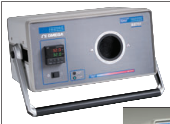
Model BB701 Hot/Cold, $2995 -17 to 148°C (0 to 300°F), 2.5" Target Plate 0.95 emissivity
